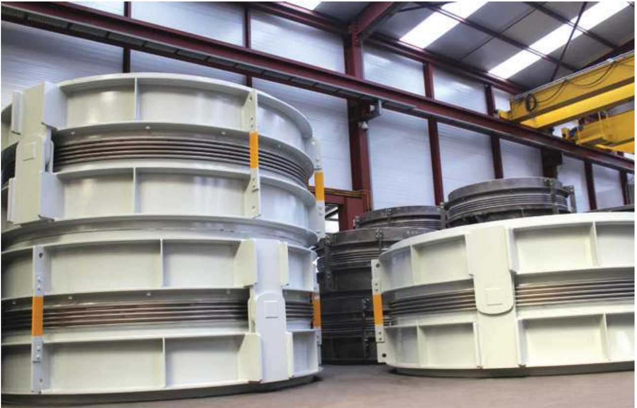
High Pressure Universal Untied Reinforced Expansion Joints for a water transfer pipeline in North Africa
