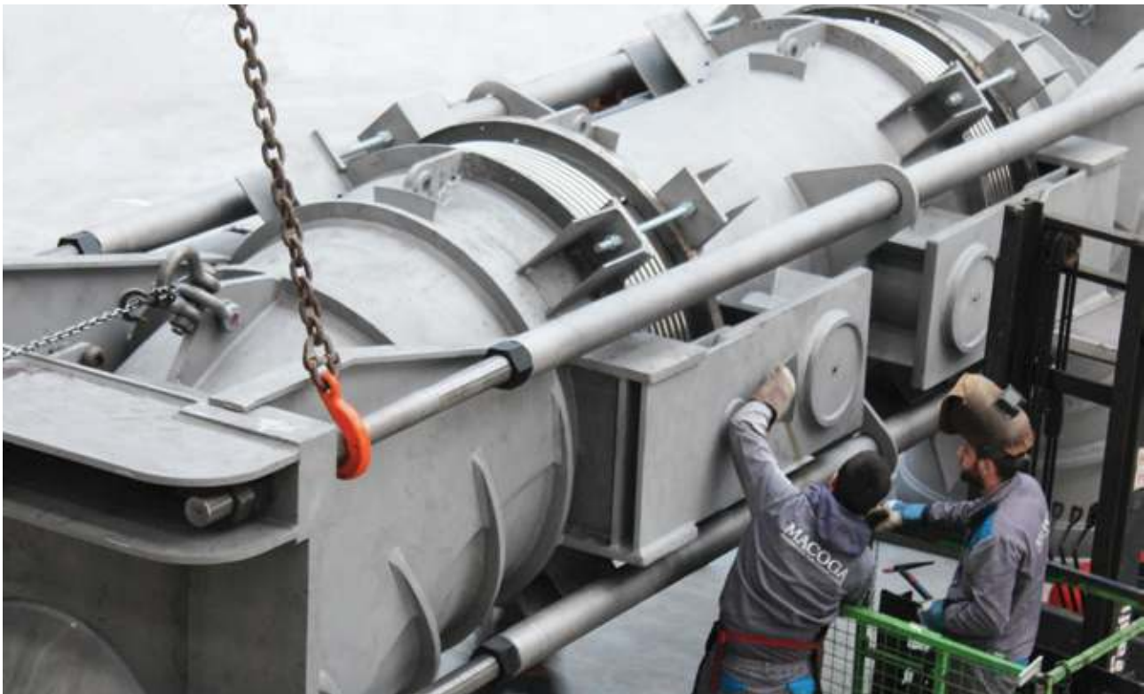
M-Lens Expansion Joints DN5900 for a cement plant.
