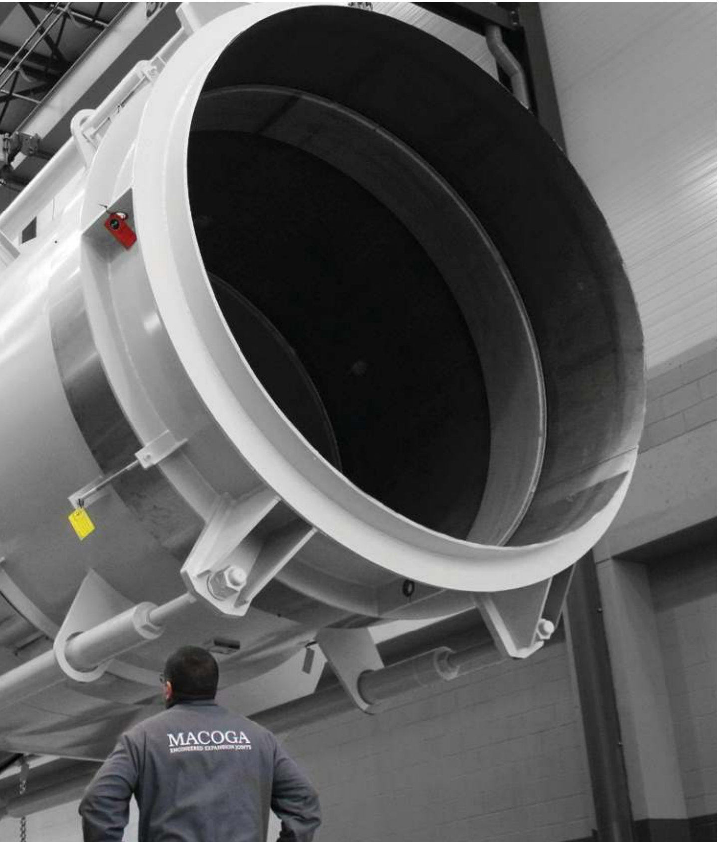
Elbow Pressure Balanced Expansion Joint for a Waste to Energy facility in the UK
